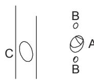
When drilling through the door, drill from both sides to avoid damaging the door.
