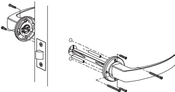
To attach furniture to the door fit the threaded spindles to one side of the backplate first then insert the square spindle with the scalloped side facing the grub screw in the handle. Then offer up to the door and fit the other handle. Screw the machine screws into the threaded spindles. Tighten the grub screws in the handles. Then add extra wood screws for strength.
